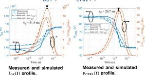
The model with the time constant obtained through  $V_{CTRL}$  presents a better fit to the measurements.
