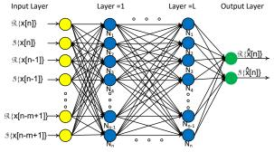
After the PA NN model is trained at the first stage, The NNs are cascaded into one NN. The cascaded NN is trained by freezing the PA model NN weights and only updating the DPD NN thus allowing it to counter the PA distortion.
