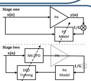
Both PA and DPD NNs are trained using a fully connected feedforward architecture. feedforward
