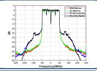
Results on a 65 nm wideband CMOS PA with a bandwidth of 2.17 GHz between 0.33-25.GHZ, using a 160 MHz 802.11ax Wifi signal. Compared to memory less backpropagation and indirect learning
