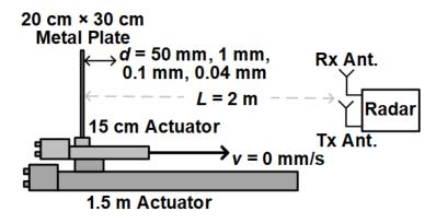
2) Vibration sensitivity under1-D constant velocity motion
