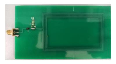
WPT: Wireless power transfer system MCR: Magnetically coupled resonators
