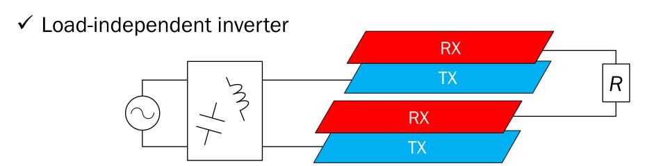
Capacitive coupler with opposite relative position of power feeding/receiving points
