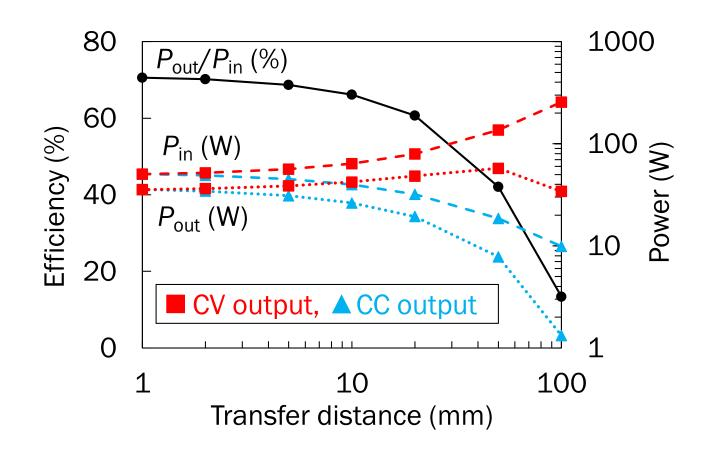
Which is suitable for the UWPT system, CV or CC operation?
