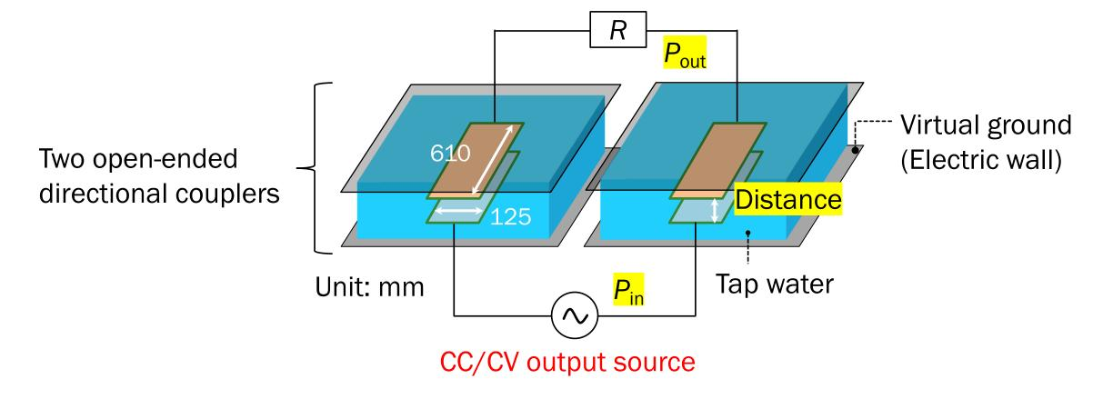
Calculation of input/output power for each operation at 13.56 MHz
