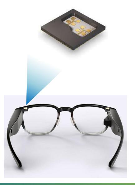
Radar chip on the **frame of a glass**
