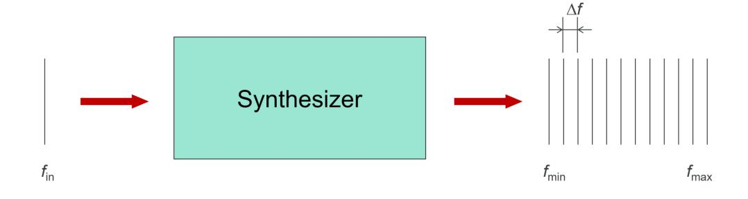
A frequency synthesizer is an electronic device that translates one (or more) reference frequencies to a number of output frequencies
