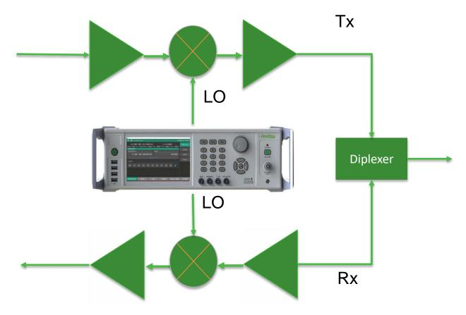
The frequency synthesizer is a key component of virtually any RF/microwave test-and-measurement, communication, and monitoring systems
