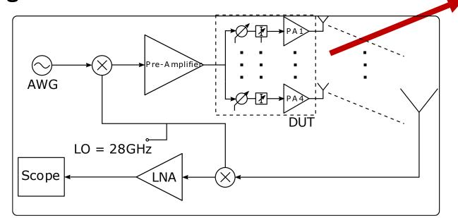
beamformer + antenna array
