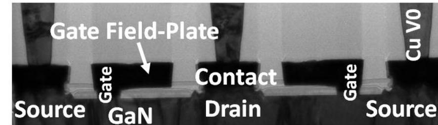
E-mode high-K GaN Transistor (Gate Field-Plate)
