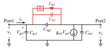
$$Y_{12} = \frac{i_1}{v_2}|_{v_1=0} = -j2\pi f \left( C_{R2} + C_{dg2} - \frac{1}{4\pi^2 f^2 L_{R2}} \right)$$
