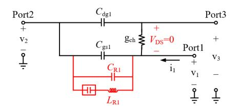
$$Y_{12} = \frac{i_1}{v_2} \Big|_{\substack{v_1 = 0 \\ v_3 = 0}} = -j2\pi f \left( C_{R1} + C_{gs1} - \frac{1}{4\pi^2 f^2 L_{R1}} \right)$$
