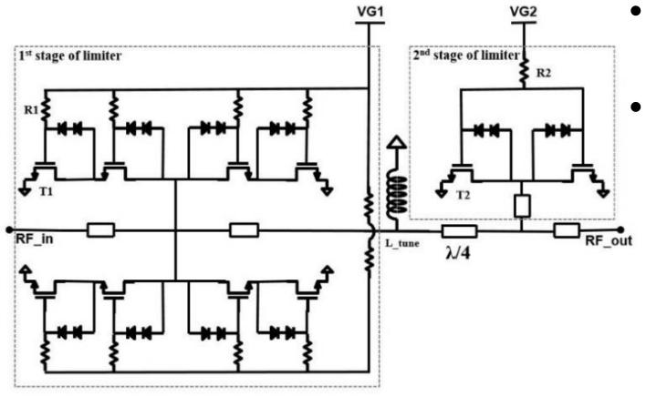
$$I_{peak} = 2\sqrt{\frac{2 P_{RF\_in}}{R_0}} \sim 6A$$
