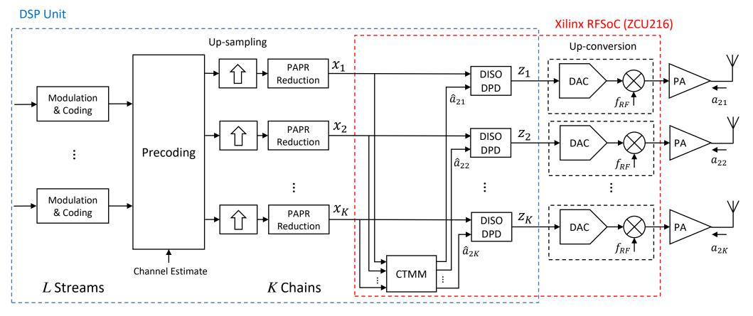
The goal of this work is to implement the DISO DPD solution for fully digital 5G MIMO transmitters on an FPGA.
