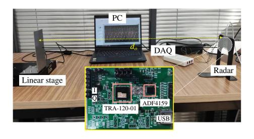
the radar is made with the radar front-end TRA-120-001 (Silicon Radar) and the PLL chip ADF4159. The I/Q signal is sampled by the data acquisition (DAQ) board (National Instruments) for post-signal processing in the computer. The radar sits around  $d_o = 56 \ cm$  away from the linear stage (Zaber X-LDM060C-AE54D12).
