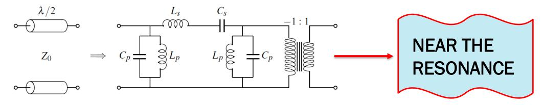
• Calculate the waveguide wavelength  $\lambda_{gi}$ , the slope parameter  $X_i$  and the characteristic impedance  $Z_{0i}$  of every *i*-th series resonator. These parameters allow us to obtain the dimensions  $a_i$  (waveguide width) and  $b_i$  (waveguide height) for each rectangular cavity (resonator).
