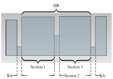
Each section and the adjacent irises are optimized to recover the response of the original <u>isolated</u> cavity.
