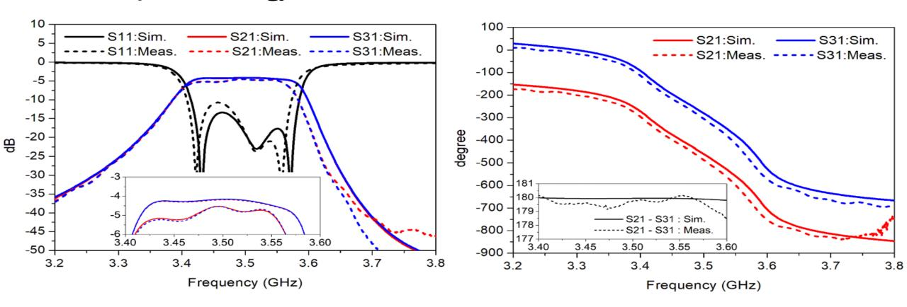
Measured IL = 1.5 dB, Amp. Imb = 0.1 dB, Phase Imb. = 0.5 deg
