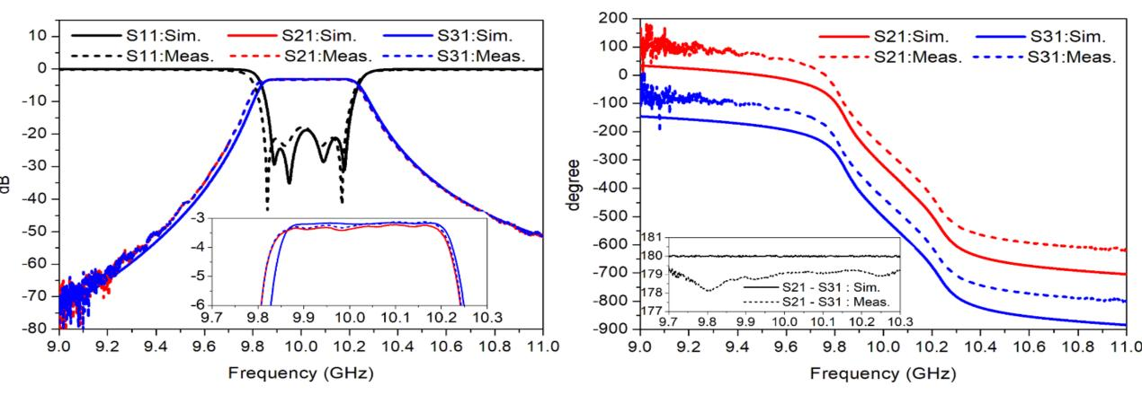
Measured IL = 0.25 dB, Amp. Imb = 0.2 dB, Phase Imb. = 1.25 deg
