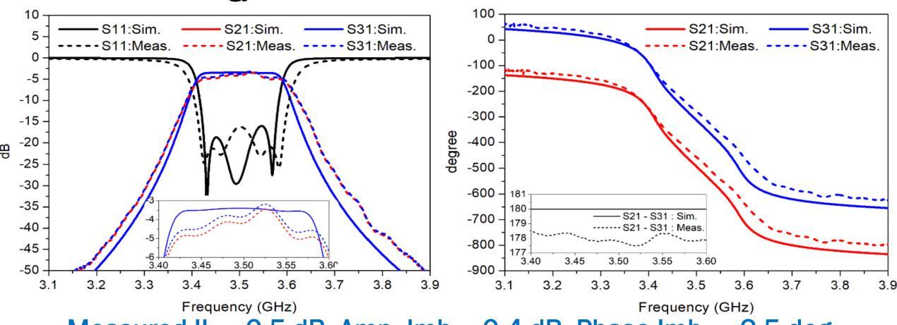
Measured IL = 0.5 dB, Amp. Imb = 0.4 dB, Phase Imb. = 2.5 deg
