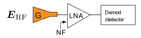
Sensitivity defined in terms of the noise figure of the LNA [W/Hz].
