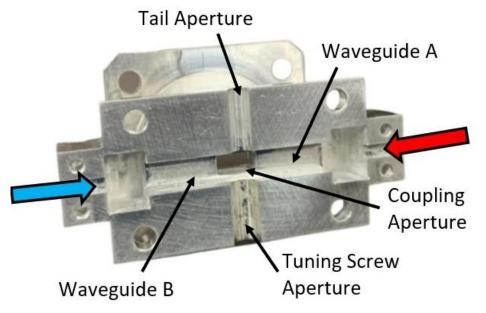
One half of the split-block machined cavity
