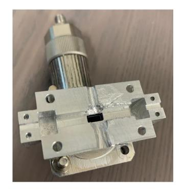
Manually drilled a taper to accommodate the bulge between the cell and the tail
