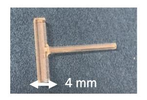
The unfilled fused silica vapor cell
