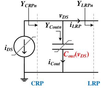
• If conventional equations are used to design PA, the harmonic tuning conditions are altered at the load reference plane (LRP).
