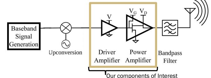
Canonically the performance of Power Amplifier (PA) determines the efficiency as measured by drain efficiency ( $\eta_D$ ) or power added efficiency (PAE) of a given transmitter.
