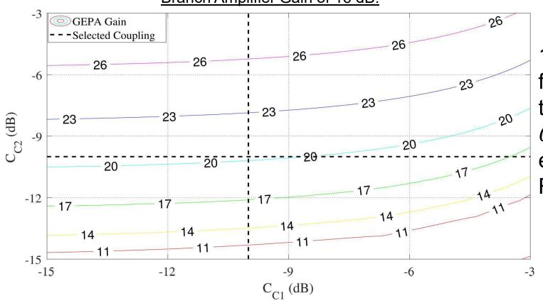
10 dB coupling factors selected in this work such that  $C_{C1} = C_{C2}$  and to ensure realizability in RO4350B.
