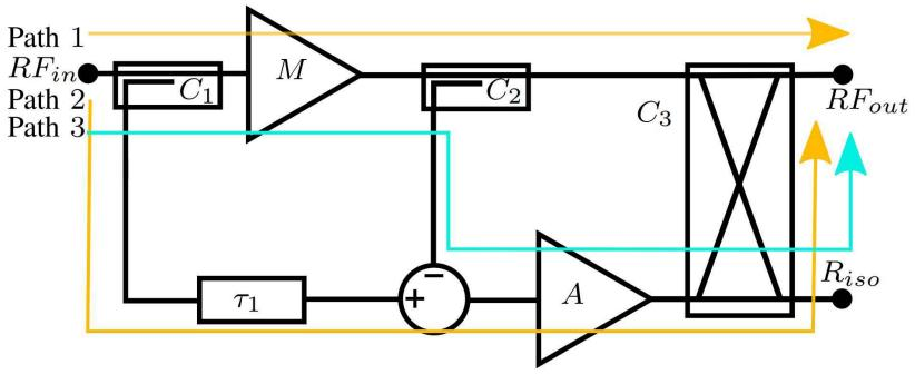
Series connection increases gain of GEPA structure!
