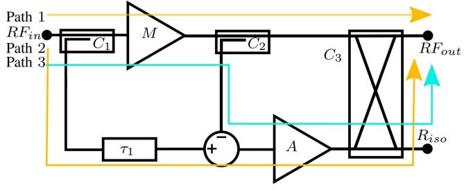
Path 1 and 2 must have equal phase to add at the output Path 3 must differ from Path 2 by  $180^{o}$
