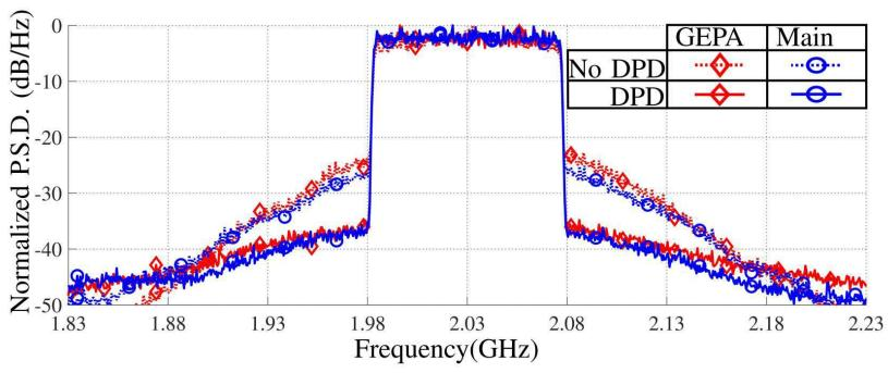
Measured output spectrum for a 100 MHz wide LTE-like signal with 10 dB PAPR
