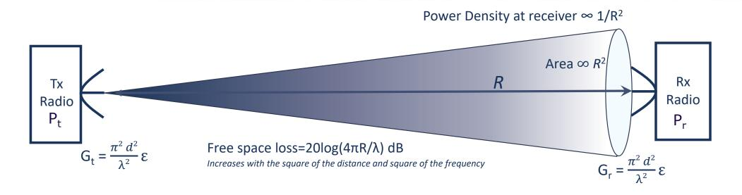
$$P_{r} = P_{t} + G_{t} + G_{r} + 20\log_{10}\left(\frac{\lambda}{4\pi R}\right) - Attenuation_{Rain} - Attenuation_{Atmosphere}$$
