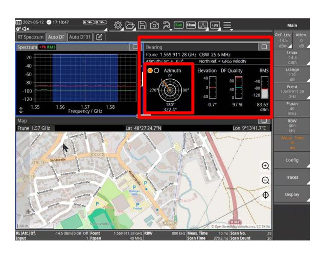
Bearing direction will be indicated inside the polar diagram and as a red line inside the map
